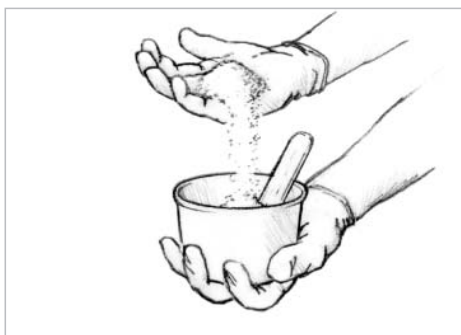
Figure 9-7 Blend in small handfuls or scoops of the appropriate filler until the desired consistency is reached.
