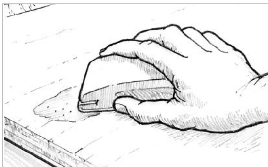
Figure 9-16 Sand the fairing material to blend with the surrounding contour.
